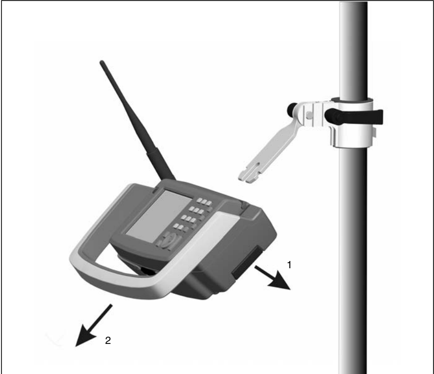
Figure 7.81 Detach Trimble Robotic Holder from standard rod adapter
