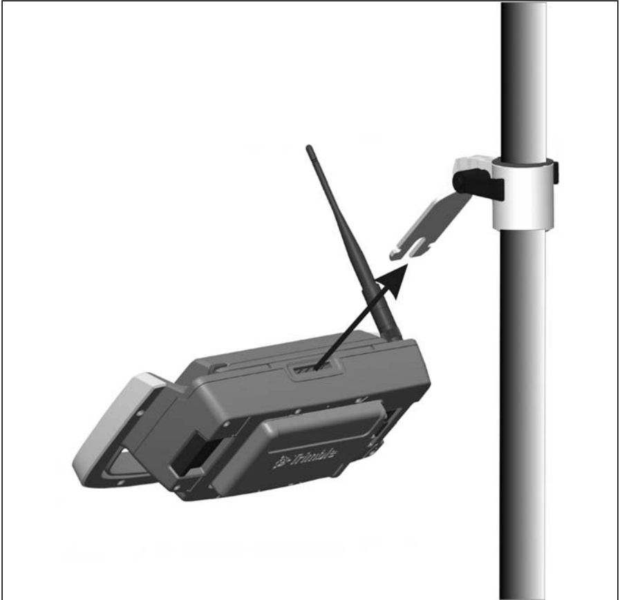
Figure 7.80 Attaching the Trimble Robotic Holder to the standard rod adapter
