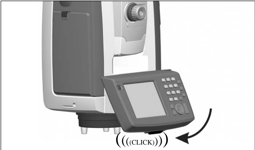
Figure 4.40 Attaching the Trimble CU
