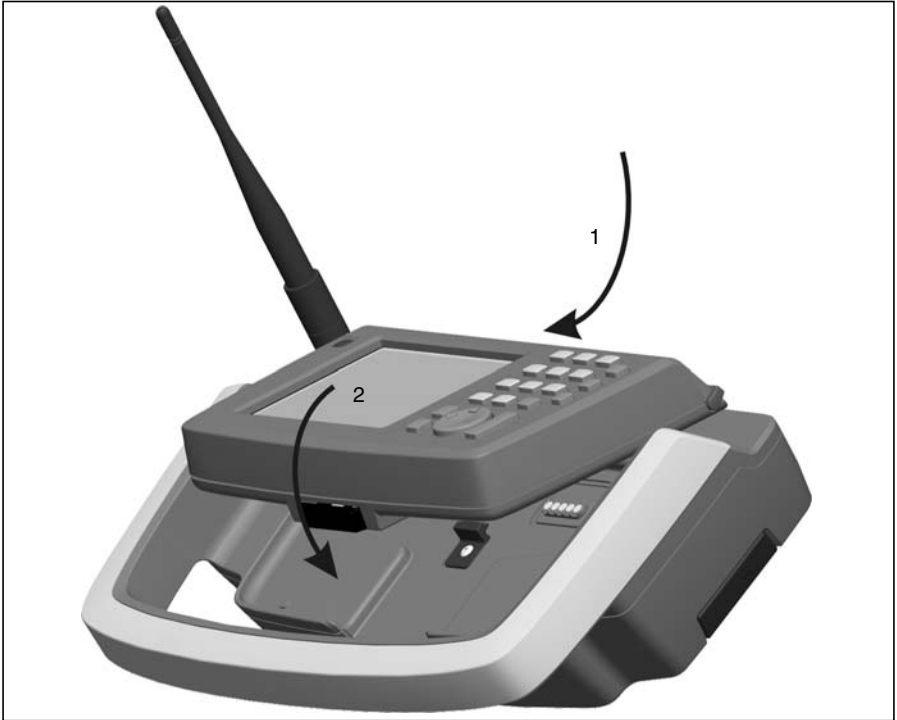
Figure 7.78 Attach Trimble CU to Trimble Robotic Holder
